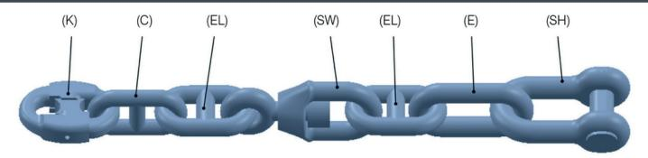
A common way to connect stud link chain to the anchor is by way of a swivel assembly allowing the anchor to rotate without twisting the chain itself. The most popular means being the swivel forerunner assembly. This is generally made up from the following components:
