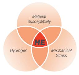
For Hydrogen Embrittlement to take place, three elements are required: a source of hydrogen, material susceptibility and mechanical stress.
