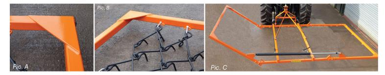
Mounted Harrows are available in widths of 6'0" through to 16'0" wide and a depth of 7'-6", frames of 10'-0" and over have manual folding wings for ease of transportation along roads and through gateways.
